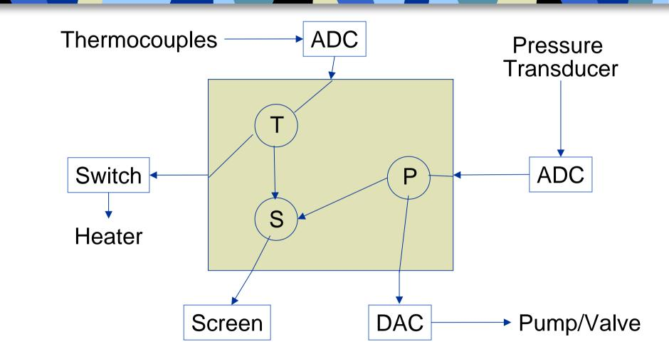
Overall objective is to keep the temperature and pressure of some chemical process within well-defined limits
