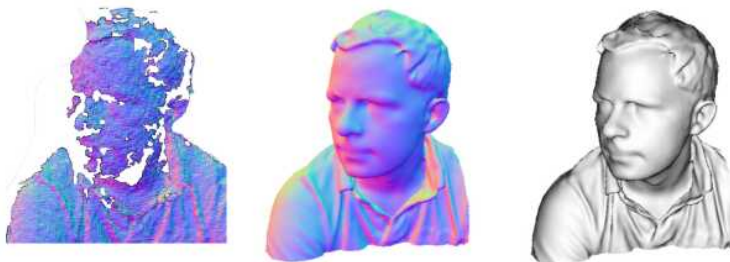
Figure 13.13 Fusing multiple depth images using the KinectFusion real-time system ( Newcombe, Izadi et al. 2011 ) © 2011 IEEE. The three images show an original (noisy) range scan, rendered as a colored normal map, and the fused 3D model, rendered as both a normal map and Phong-shaded.
