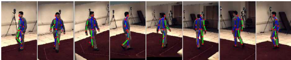
Figure 6.25 Pose detection using random forests (Rogez, Rihan et al. 2008) © 2008 IEEE. The estimated pose (state of the kinematic model) is drawn over each input frame.
