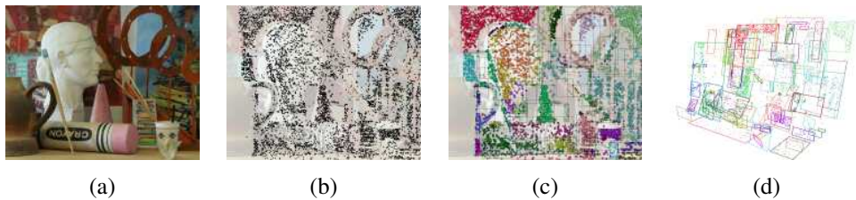
Figure 12.12 Stereo matching using local plane sweeps (Sinha, Scharstein, and Szeliski 2014) © 2014 IEEE: (a) input image; (b) initial sparse matches; (c) matches grouped by slanted planes; (d) 3D visualization of planes and grouped features.
