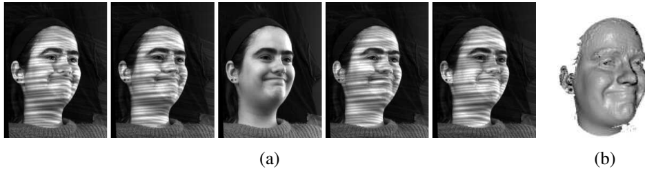
Figure 13.10 Real-time dense 3D face capture using spacetime stereo (Zhang, Snavely et al. 2004) © 2004 ACM: (a) set of five consecutive video frames from one of two stereo cameras (every fifth frame is free of stripe patterns, in order to extract texture); (b) resulting high-quality 3D surface model (depth map visualized as a shaded rendering).
